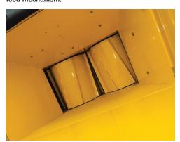
**SMOOTH FEEDING.** Vertical feed rollers with helical clears help hold material firmly to the infeed table which reduces vibration, shock and structural loading to the rear of the machine.
