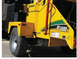
**NEVER GET STUCK.** The BC1500 comes with 40.1cm floatation tires as standard. Effortlessly drive over soft terrain like loose dirt with minimal soil disruption.
