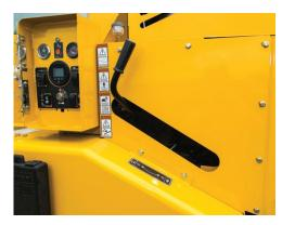
**EASY ACCESS.** The hinged thermoformed plastic engine enclosure design helps with easy access to maintenance points and limited noise.
