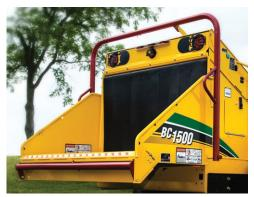
**OPERATOR SAFETY.** The four-position upper feed control bar enables the operator to stop the feed rollers and select forward/reverse. The patented bottom feed stop bar is strategically located so an operator's leg can strike the bar and shut off the feed mechanism.
