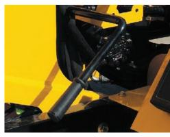
**CLUTCHLESS PTO SYSTEM.** Prevent premature wear to the belt-drive system using the clutchless PTO system, which prevents high-speed engagement of the cutter drum.
