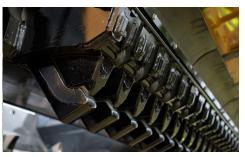
**DOUBLE-ENDED COMB TEETH.** The LS3600TX has individual bolt-in comb teeth that have two usable edges. This helps extend the life of your teeth and minimize wear costs.
