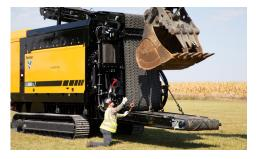
**SERVICEABLE BELLY CONVEYOR.** The belly conveyor can be removed without detaching the discharge conveyor – allowing for minimally invasive service.
