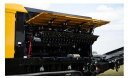
**FULL ROTOR ACCESS.** The hydraulically operated side door provides full exposure to the rotor, comb and belly conveyor to minimize maintenance time. The service area has been designed to allow you to perform maintenance without overhead obstructions.
