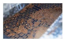
**BALANCED ELLIPTICAL SHAKER MOTION.** This motion provides a more even conveyance of solids across the shaker decks and improves the ability to carry lower gravity solids, such as clay, over the shaker screens.
