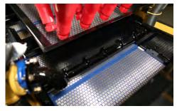
SCALED SHAKER DECK. This cutting-edge design features a proportioned double-deck shaker that gives critical access and visibility to the bottom deck without sacrificing overall screen square footage.
