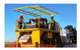
SEAMLESS OPERATION. The R250c reclaimer is a modular mud recycling machine that can pair with a variety of directional drills and mud pumps on a jobsite. Its mobile nature allows the machine to move where you need it, when you need it.
