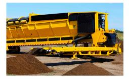
**RADIAL STACKING CONVEYOR.** Simple stacking conveyor with 180° arc increases the amount of material being stacked on the ground. Adjustable stacking height aids with dust control and helps avoid material being blown away.
