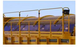
STAINLESS STEEL SCREEN OPTION. Stainless steel screens offer increased durability and help reduce the amount of screen blinding when working with wet or corrosive materials.
