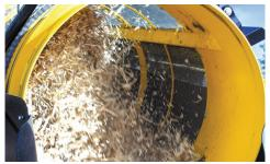
**HIGH PRODUCTION.** The tensioned screens around the drum add rigidity, allowing use of smaller-gauge wire — which helps increase production capacity and enable processing of wetter material.
