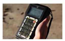
ADVANCE CONTROLS. Operators can control the machine through either the Vermeer DP10 display mounted on the control panel, or through a handheld transceiver remote.
