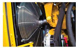
**OPERATING EFFICIENCY.** With features such as a hydraulically driven variable flow and reversing Flexxaire cooling fan, the TG5000 is built with operating efficiency top of mind. The fan adjusts the pitch of the blades based on temperature, which can increase the power available to the mill for better processing efficiency.
