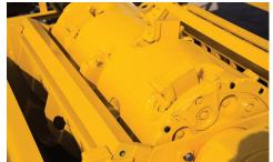
**OPTIMAL CUTTING PERFORMANCE.** The new Series III duplex drum is built off the proven cutting performance of previous Vermeer duplex drum designs, and makes maintenance more convenient with enhancements such as an independently secured wedge system and enhanced drum balancing.
