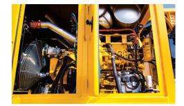
**ENGINE POWER.** The TG5000 is powered by a 540 hp (403 kW) Caterpillar C15 Tier 4 Final engine. A Tier 3 engine option is available for lesser-emission regulated countries.
