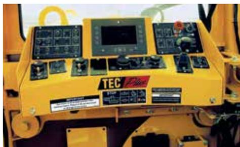
**TEC® PLUS ELECTRONIC CONTROL SYSTEM.** The operating system communicates with multiple control modules located throughout the machine for real-time performance data and advanced troubleshooting capabilities.
