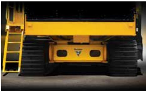
**MOBILITY AND STABILITY.** The T1655III dual tracks and low center of gravity allow for easy maneuverability and stability over the changing and diverse surface conditions.
