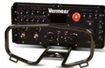
**FULL FUNCTION REMOTE CONTROL.** The T1655III is available with a wireless remote control that can provide full operator function remotely.
