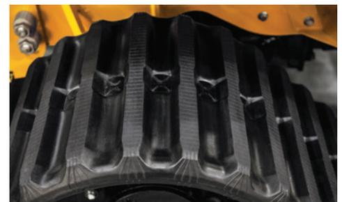
**QUAD TRACK SYSTEM.** The quad track system offers improved floatation, reduced surface damage and increased tractive effort. Four-wheel steer and crab steering are functional with both quad track and tire options.
