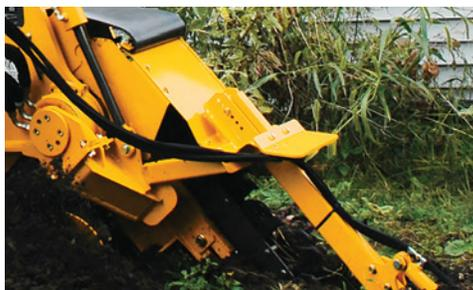
**MAKE SENSE OF YOUR TRENCH.** When difficult conditions are encountered while trenching, causing a sudden drop in engine speed, the TrenchSense™ electronic control system automatically pauses the forward motion of the tractor to prevent engine shutdown and recalibration of the machine controls. Once preset engine and trencher speed recovers, forward AutoCreeper resumes. The sequence occurs within seconds and requires no operator adjustment.
