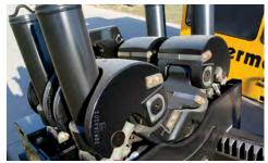
ROBUST AND POWERFUL. Robust vise design uses a planetary gear for breakout power.
