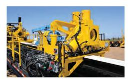
STAY ON SCHEDULE. A floating vise allows the breakout system to clamp the rod fully during breakout, helping to prevent rod wrap and keep your crew on schedule.
