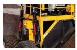
PRECISE CONTROL. Equipped with independently controlled lift cylinders for thorough aeration of the compost pile.
