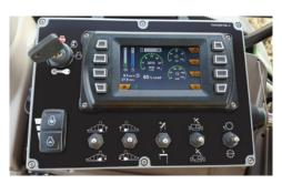
**CONTROL SYSTEM.** Operators can monitor and control the machine from the comfort of the tow vehicle. Changes can be made on the fly as the unit goes through the windrow.
