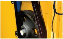
**RELIABLE COMPONENTS.** The poly-synchronous belt drum drive helps reduce maintenance and offers efficient transfer of power.
