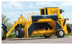
**CONVENIENT TOWING.** An optional low-speed transport kit makes converting between work and transport modes quicker and easier. The CT616 can be changed from transport to operating mode using machine hydraulics.
