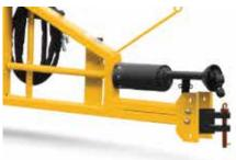
**CONVENIENT TOWING.** An optional low-speed transport kit makes converting between work and transport modes quicker and easier using tow-tractor hydraulics and simple hand tools.
