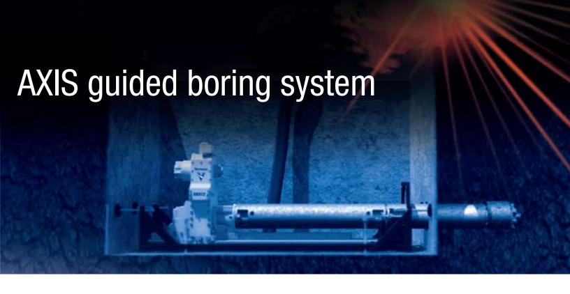
Located in the launch pit is the core of the AXIS system, which is made up of the rack, drill casings, drill head and pipe laser.
