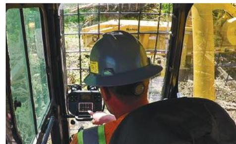
**CONVENIENT CONTROL.** The transceiver remote is equipped with the machine control menu, providing the ability to supply the user with machine-operating information to monitor the machine's health, and a fault log.
