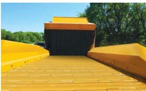
**CONVENIENT FEEDING.** The HG6800TX features low sidewalls to aid in feeding whole trees and other larger material with less restriction, reducing the number of user interactions with the material.
